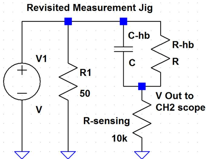
Once the circuit was wired up on the bench, the phase of the voltage across  $R_{sense}$  relative to the phase of the generator voltage was evident, measured at 52 degrees at 1 MHz. Yup folks, we have an RC circuit with a classic phase shift.
