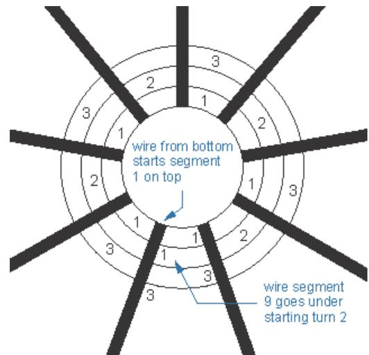
Windings of the first few turns are displayed in picture 2. The winding starts from the back of the interior center; hence the first and all odd segments of the first turn will show on the top side as noted by "1." The last segment of turn 1, segment 9, comes out on top and zig-zags over to become turn 2, where it goes underneath the form again. The following segment of turn 2 is then on the top as noted, and so on.
