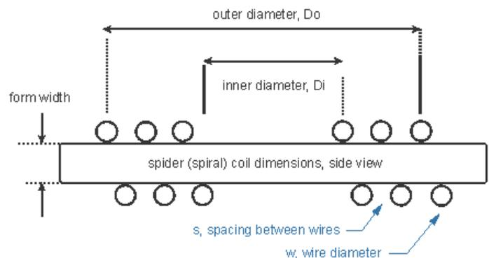
of the coil, the spider coil approaches the same dimensions as a flat spiral coil wound on one side of the form. Thus, the equation for the spiral coil can be used when winding the spider coil.
