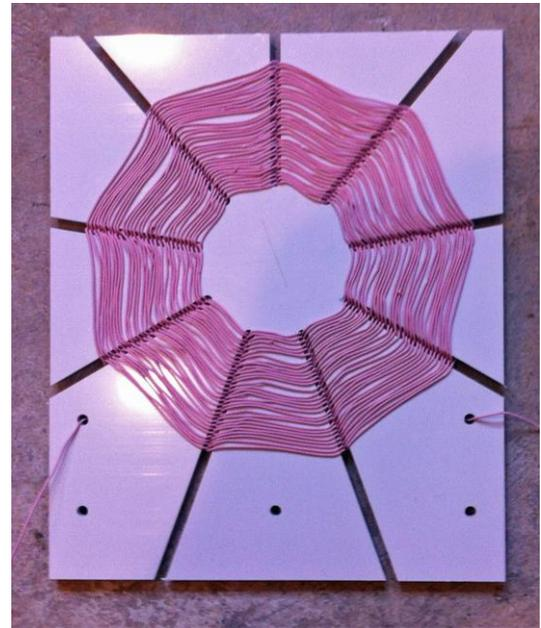
Spider web and basket weave coils will produce a stronger signal than their cousin, the standard close wound cylindrical, for a given input signal. This is accomplished by separating adjacent windings by the thickness of one winding. This separation reduces the proximity effect between wires, wherein the closer they are a current in one will increase the resistance of the other.
